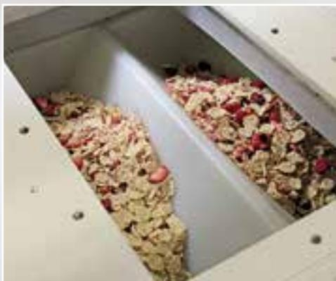
*Feed point with silicon seal*
