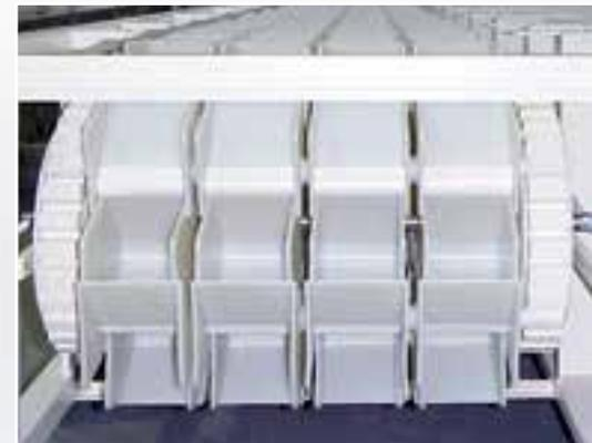
Multiple bucket belt at the tensioning unit
